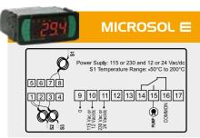
Differential thermostat for solar heating with three sensors\* that controls the water circulation pump based on the temperature differential between the solar panels and the thermal tank, or swimming pool. It has functions to ensure the efficiency of the heating system, prevent the freezing of the pipes during winter and control overheating.
